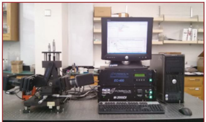
Figure 5. The spectroscopic ellipsometer in our laboratory (from the J.A. Woollam company).
